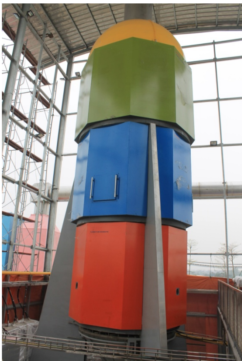
- Plasma Pyrolysis Incinerators System, in DongAnh MSW Treatment Plant (500TPD) -
