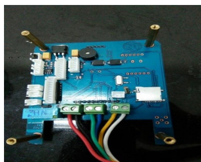
Fig. 10. The PCB after welding process
