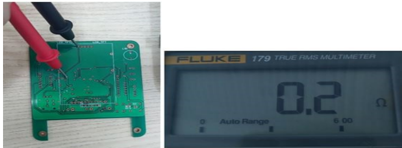
Fig. 8. Testing the impedance of the circuit lines using VOM meter
