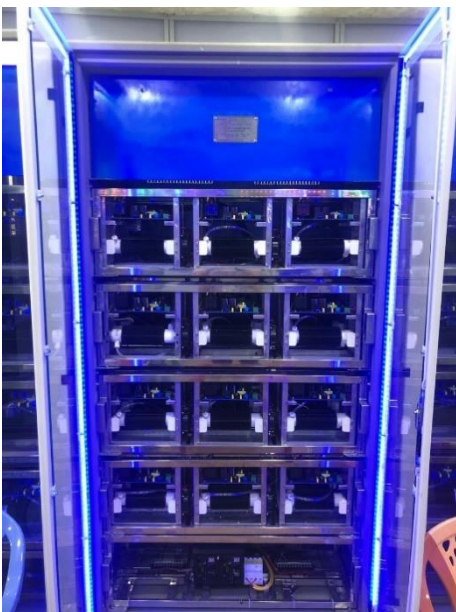
Tủ Plasma Ozone Generator
